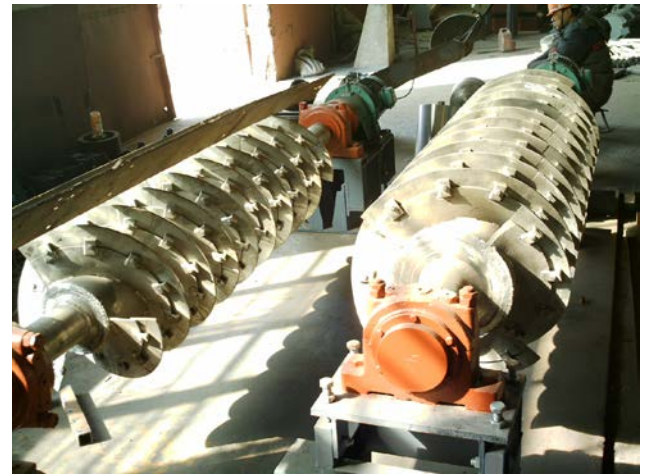
Cake discharge screw conveyor arms
